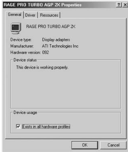
FIGURE 1.3 The Windows Properties dialog box for the video card may provide information on the video chipset manufacturer.
