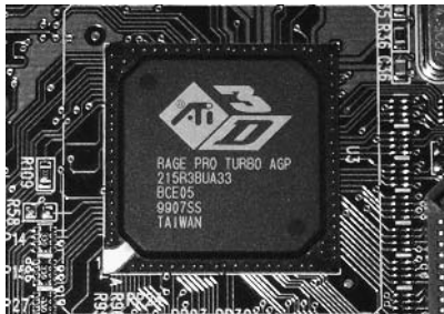
FIGURE 1.4 Markings on chips can help identify the chipset for X.
